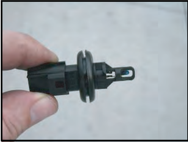
Sensor Installed in Grommet
