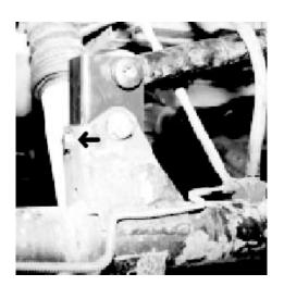
14. Check Brake Line Length, if they seem too short, longer stainless steel DOT Approved lines are available from Rugged Ridge. A driveline vibration may occur. If so, a transfer case lowering kit from Rugged Ridge should be installed.
