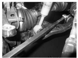
**13.** Place a jack under the lower control arm. Raise the lower control arm to reattach the lower ball joint bolts. Torque the ball joint nuts to OEM specs.
