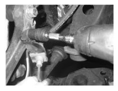
4. Detach all brake hose brackets from the steering knuckle and upper control arm. On vehicles with ABS, remove the front wheel speed sensor-retaining bolt and detach the sensor from the steering knuckle. 5. Let the sway bar swing down out of the way. Failure to do this will prevent the removal of the strut assembly.
