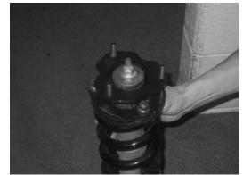
**11.** Place strut back into upper strut mount. Tighten provided nuts snug with wrench or ratchet (after install, you will torque to OEM specs).
