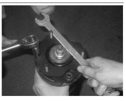
\*\* Caution: Use the factory nuts with the factory studs\*\*10. Run down nuts snug with end wrench. Torque to OEM specs.
