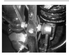
2. Using a 17mm ratchet, remove the nut from the bolt connecting the front sway bar link and the steering knuckle on both sides of the vehicle. HINT: If the ball joint turns together with the nut, use a 6 mm hex wrench to hold the stud.
