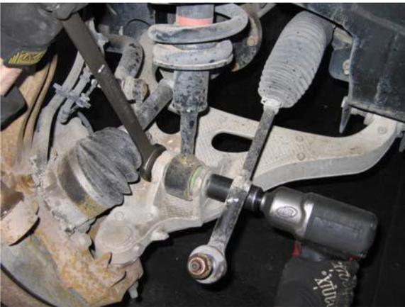
8. Remove the strut assembly.
