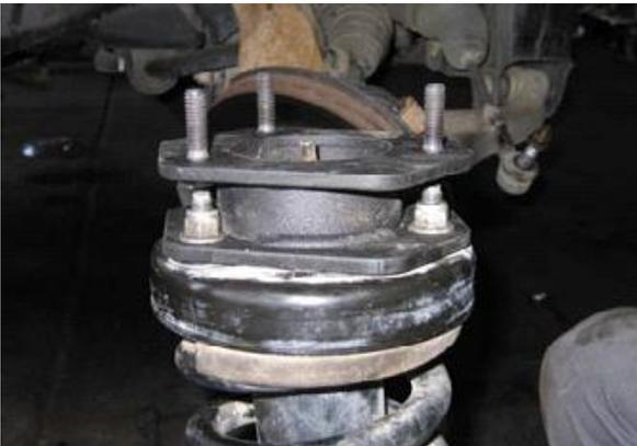
10. Run down nuts snug with end wrench. Torque to OEM specs.
