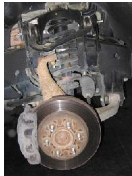
2. Remove the upper strut mounts with a 15-mm wrench of socket. You will need a socket to remove the far strut mount.
