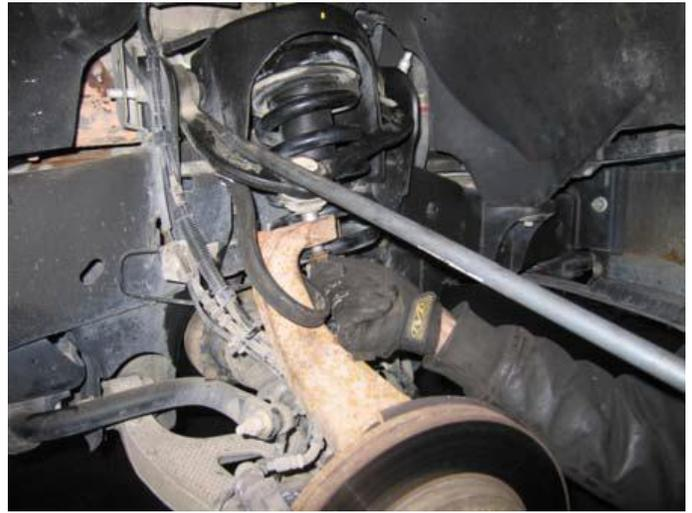
14. Reattach the tie rod end. Torque to OEM specs.
